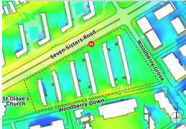
01a Solar exposure - existing conditions
