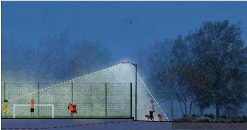
Angled lighting to reduce light spill onto the New River
